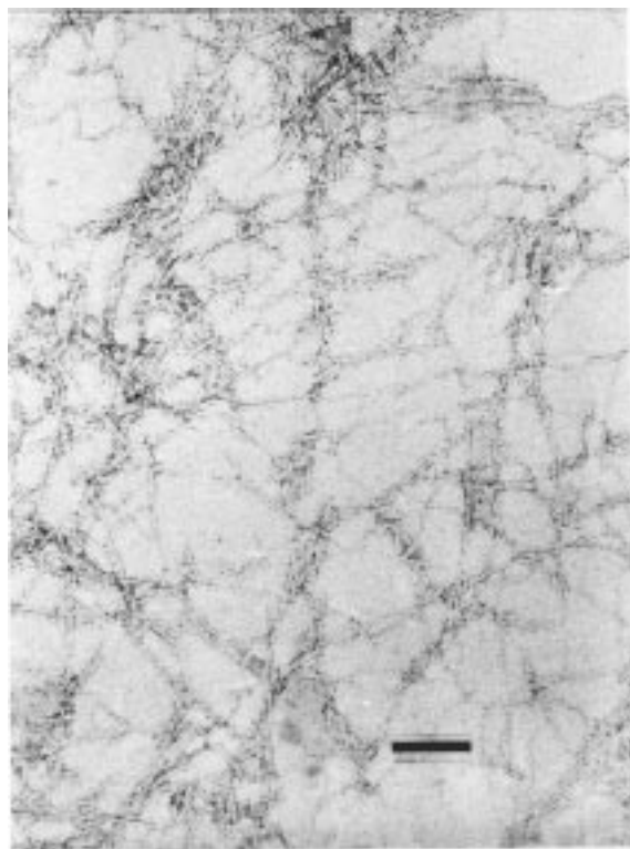
Figure 3. Electron micrograph of fibrils formed by the synthetic peptide \text{Ac}(\text{GSGAGA})_2\text{NH}_2 , an analogue of silk II, crystallized from DMSO. Similar fibrils were obtained by evaporation of the DMSO solution on a Formvar coated grid. Bar = 100 nm.
